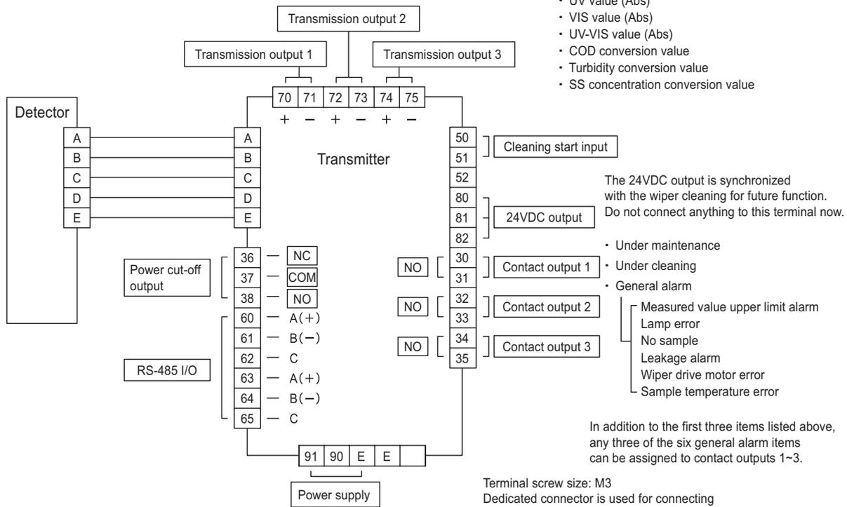
The 24VDC output is synchronized with the wiper cleaning for future function. Do not connect anything to this terminal now.
