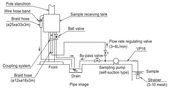
● Sampling type (mounted on aluminum frame)
